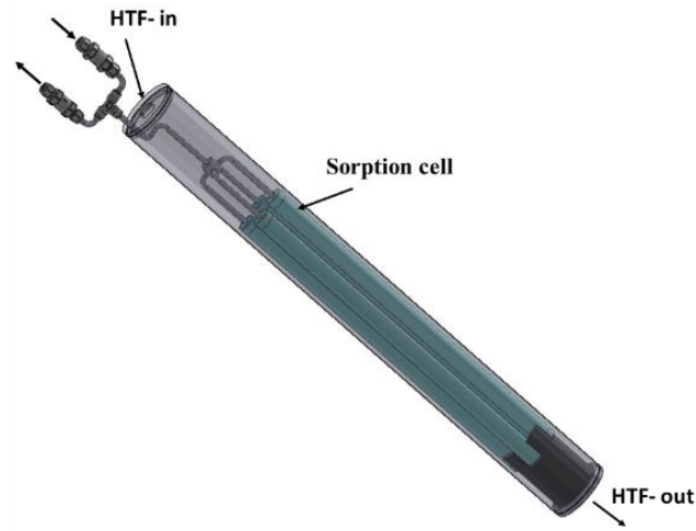
Figure 6: A CAD model of the type-D' sorption cell.
