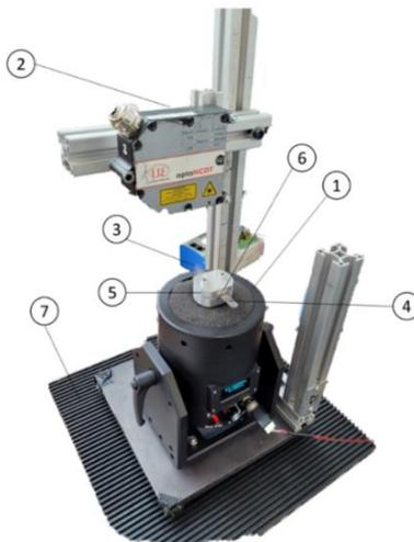
**Figure 1: Test setup to measure the bending fatigue of Reed Valves**
