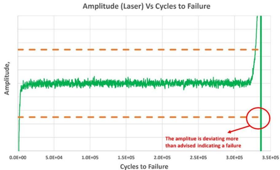
**Figure 2: Amplitude Control in Software and detection of crack in Valve Reed**
