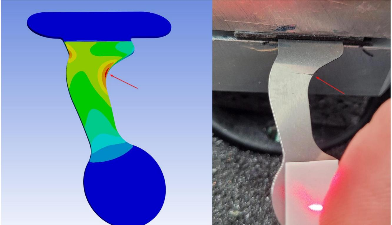
Figure 5: Stress from FEA and crack location from test failure
